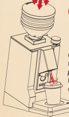
Once the coffee no longer comes out of the outlet chute, keep the tab closed and push the Blow Up System applied on the bean hopper, for the time necessary to clean the grinding chamber
